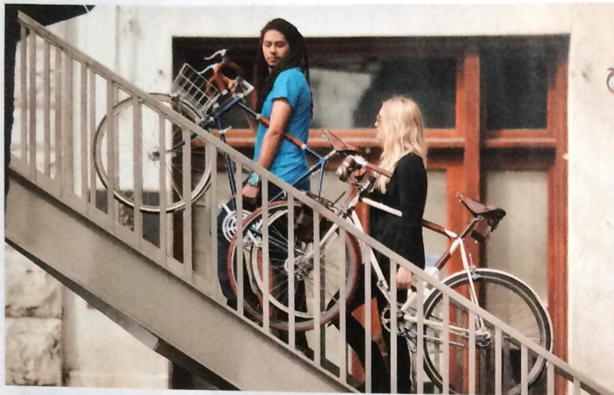
Leather frame handles, dubbed Little Lifters, reduce strain by allowing riders to carry a bike much like a grocery bag or a briefcase.
