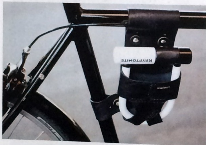
ABOVE: This frame-mounted U-lock holster cradles a bike lock to prevent rattling.
